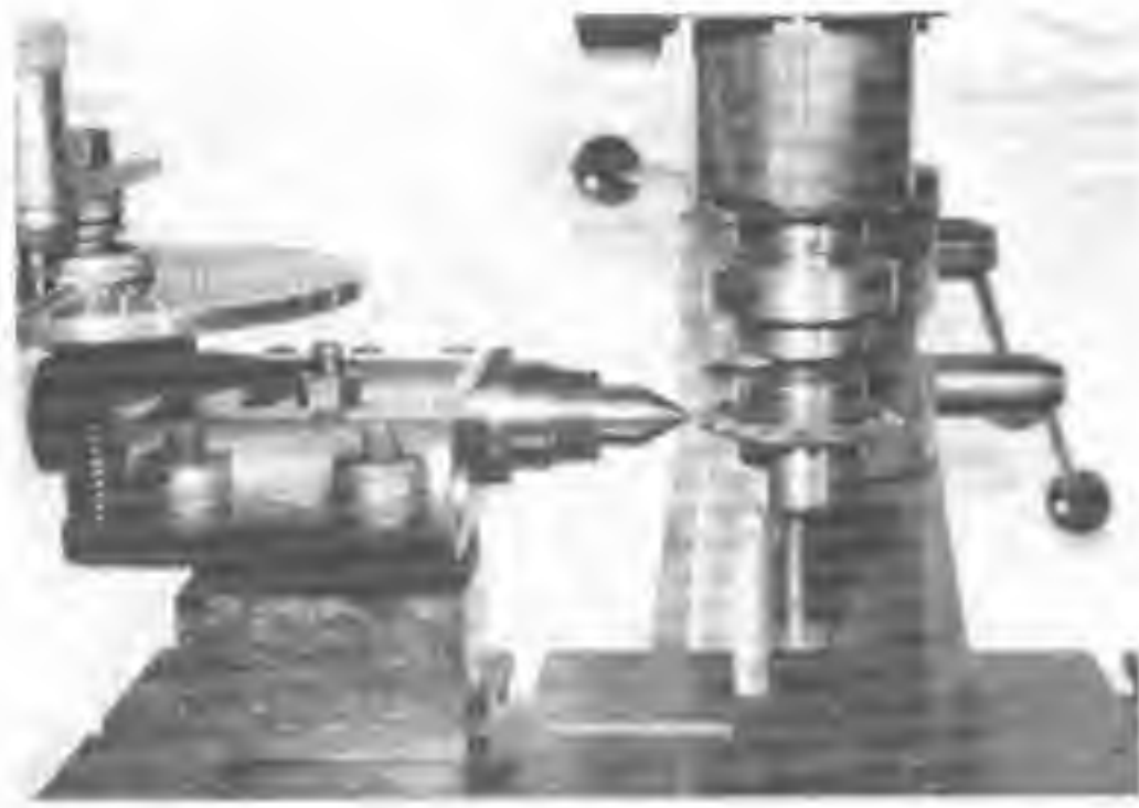
Fig. 68 Centring the cutter on a vertical milling machine.
